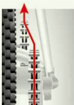
Fig. 46. Sprockets are not aligned correctly @Gates
